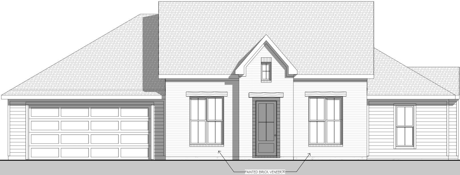
FRONT ELEVATION 9'-1", 10'-1", 12'-1", 13'-1" PLATE HEIGHT 7:12, 14:12 ROOF PITCH
