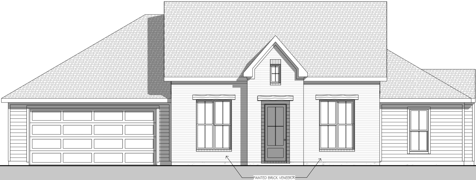
FRONT ELEVATION 9'-1", 10'-1", 12'-1", 13'-1" PLATE HEIGHT 7:12, 14:12 ROOF PITCH
