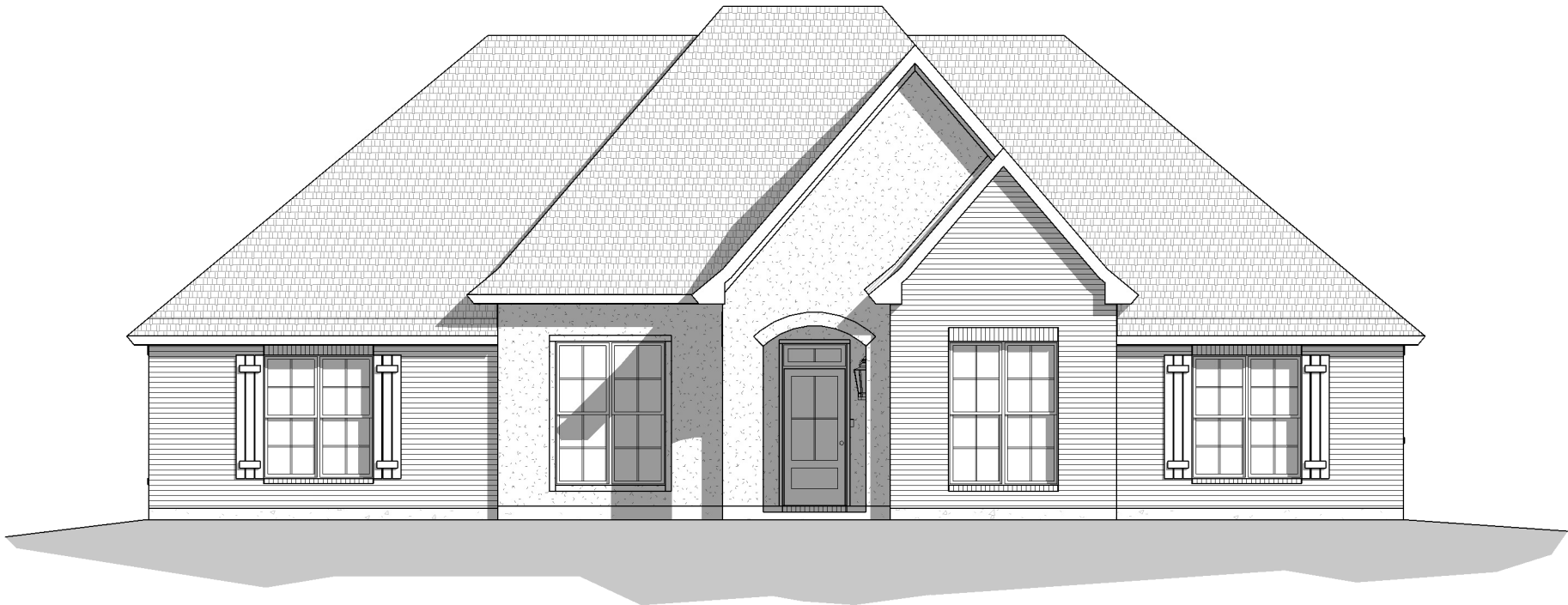
FRONT ELEVATION 9'-1" # 11'-1" PLATE HEIGHT - 9' # 11' CLG. 10:12, 14:12 ROOF PITCH
