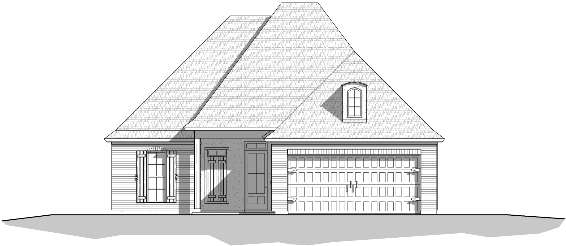
FRONT ELEVATION 10'-1"; 10'-8"; 11'-8" PLATE HEIGHT 10'; 11' CEILINGS 4:12; 9:12; 12:12 ROOF PITCH
