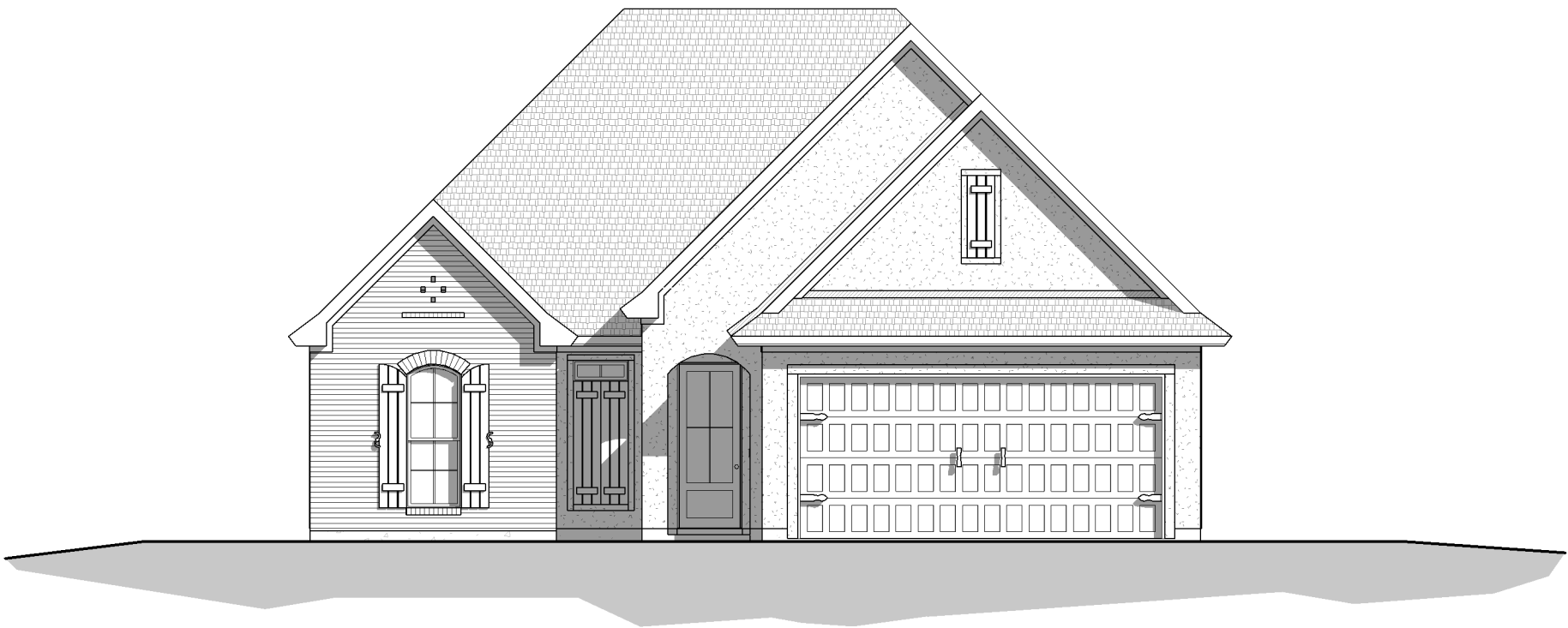
FRONT ELEVATION 10'-1"; 10'-8"; 11'-8" PLATE HEIGHT 10'; 11' CEILINGS 4:12; 9:12; 12:12 ROOF PITCH
