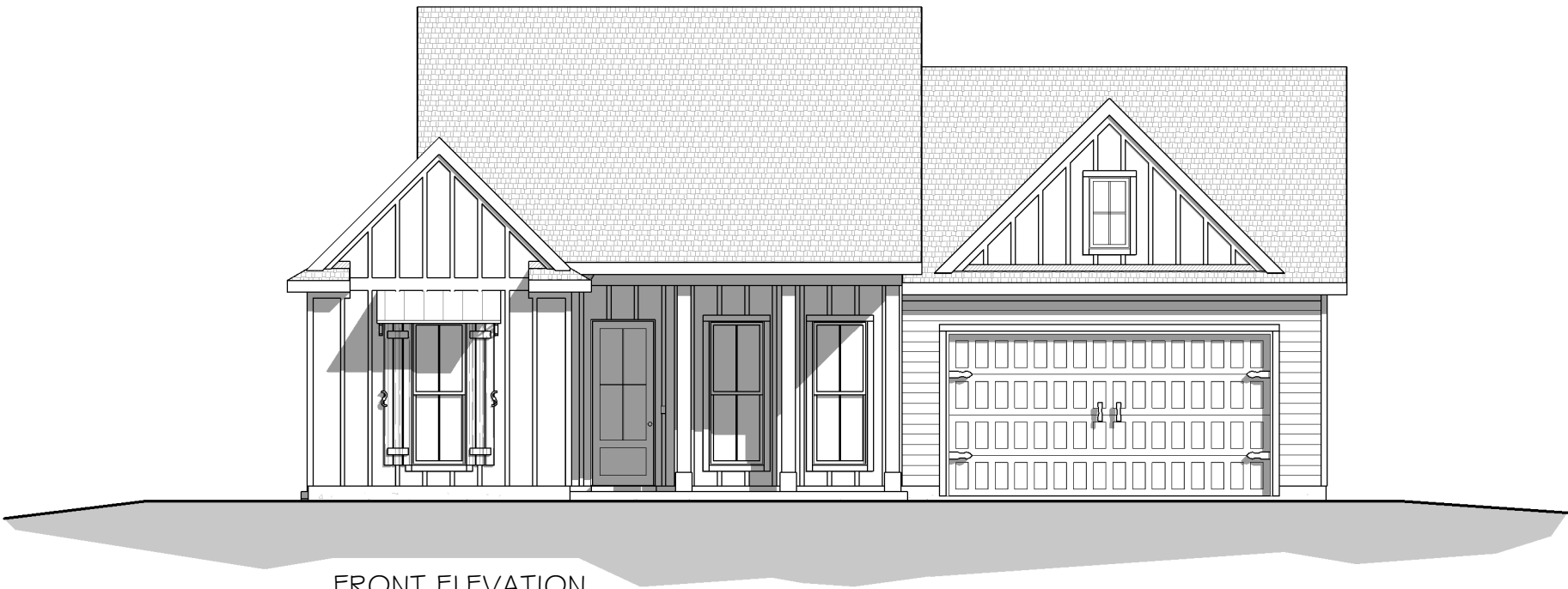
FRONT ELEVATION 9'-1" # 10'-1" PLATE HEIGHT - 9' # 10' CLG. 9:12 # 12:12 ROOF PITCH
