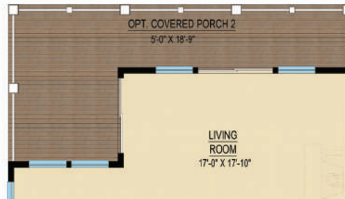
PARTIAL SECOND FLOOR PLAN OPTIONS SHOWN: SECOND SLIDING GLASS DOOR ILO CENTER WINDOWS W/ COVERED PORCH 2
