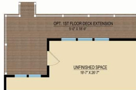
PARTIAL FIRST FLOOR PLAN W/ OPT. 1ST FLOOR DECK EXTENSION
