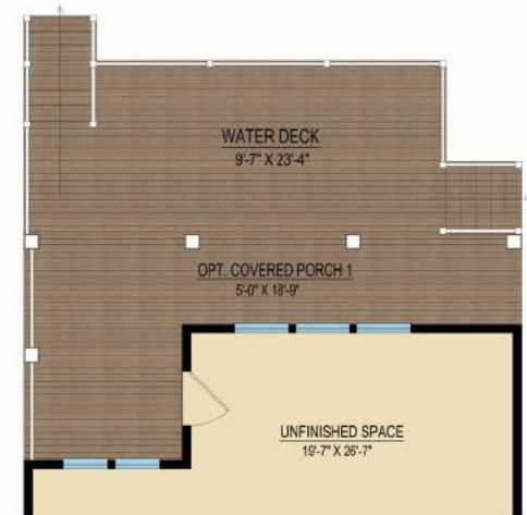
PARTIAL FIRST FLOOR PLAN W/ OPT. COVERED PORCH 1 AND OPT. WATER DECK
