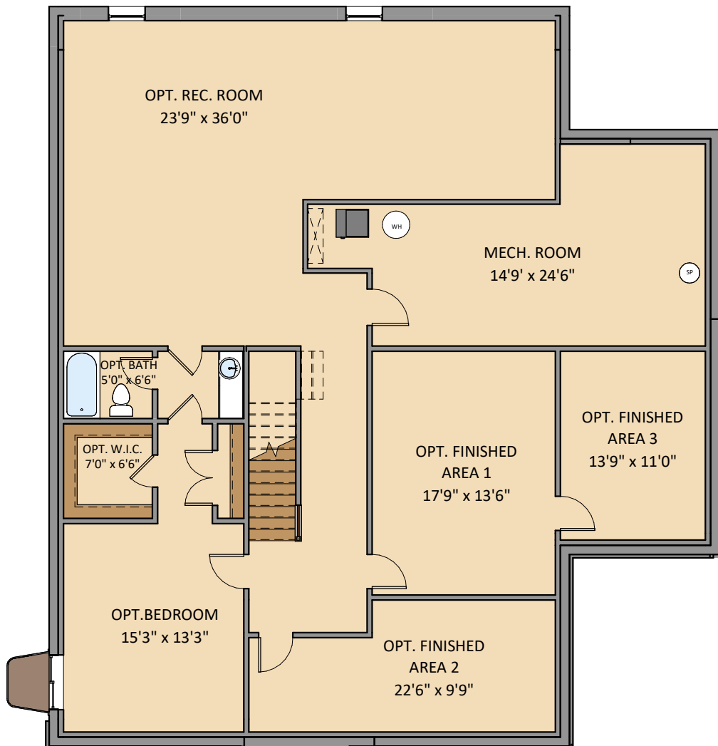
Finished Basement Plan with Buried Condition
