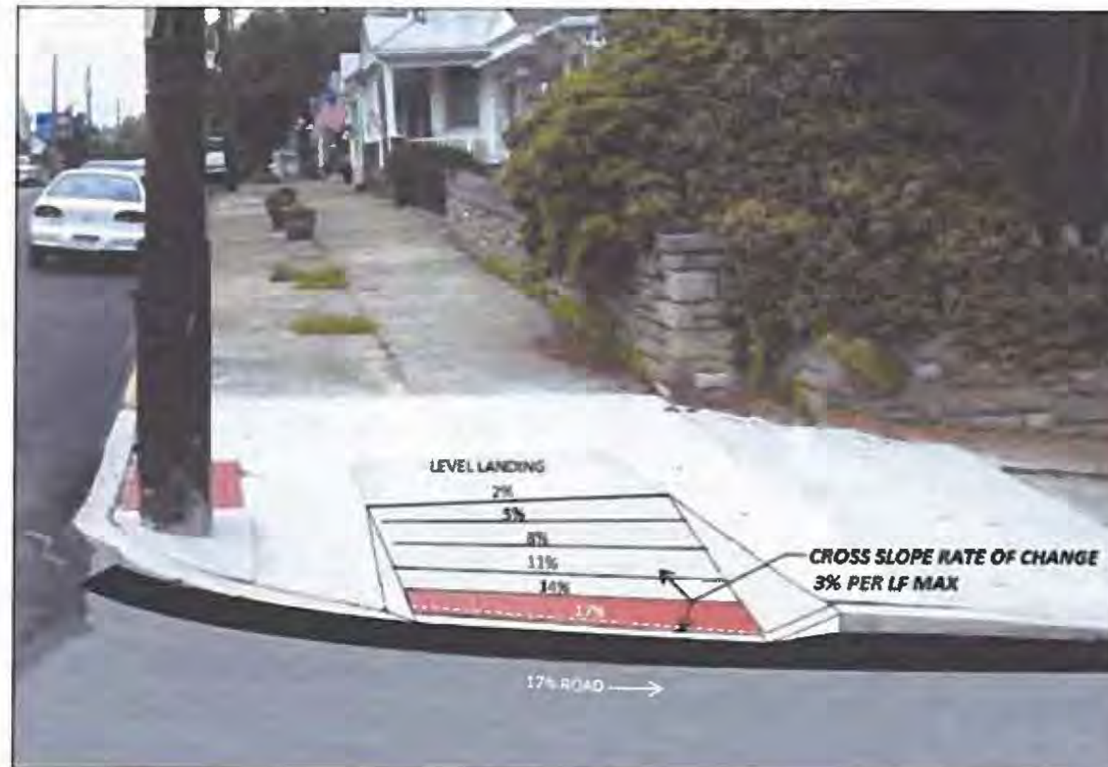
RAMP CROSS SLOPE TRANSITION TO MATCH ROADWAY PROFILE SLOPE * SLOPES SHOWN ARE FOR ILLUSTRATION ONLY.
